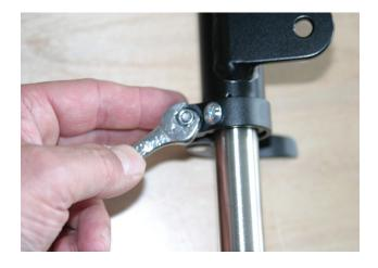
Unscrew the female screw on the clamp.
