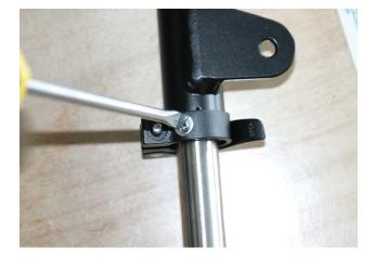
Unscrew and take out the screw in the clamp.
