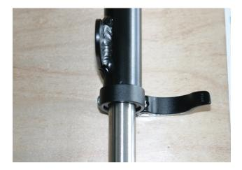
Loose the clamp on the handlebar.
