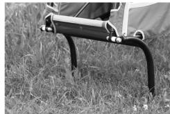
This is how it looks like when the kickstand is installed. Included in the equipment of the model TAHOE (the pure trailer), by the other two models is the kickstand an option (accessory).
