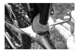
11. Attach the drag bar to the adapter use the long screw enclosed and the black plastic quick-release lever. Tighten up the lever, then also the screw (with the spanner).
