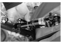
6. Put the big wheel on - first put the disc on the wheel between the calipers of the brake. Then press the button on the axle, push it in the swinging fork and in the nave of the wheel.
