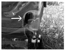
This is where you should click up/ forward the axle with the two small wheels to the frame.
