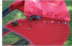
Roll the roof carefully in to the scroll. Use the two straps on the each side of the scroll to attach it to the cab.
