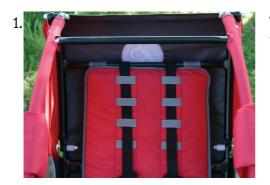
The lower "comfortable" position - the seat hangs on the lower tube.
